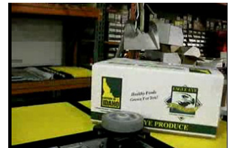
High efficiency drive uses only 25 watts to carry 200 lbs.
