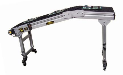
**Product Description:** 115 Volt AC motor driven chain belt conveyor with 3/8" high vertical flights on 3/4" centers. Variable speed control to match your exit speed. Static dissipative belting is custom molded by **SmartMove**® with "snap-together" features and proprietary self-lubricating additives that virtually eliminates belt wear and maintenance. Safe, clean and simple!
